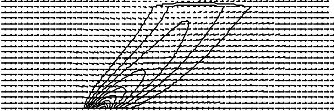
Figure 4. At high enough horizontal velocity of the water, the induced swirl flow is broken.  $V_{hor}=0.2$ .
