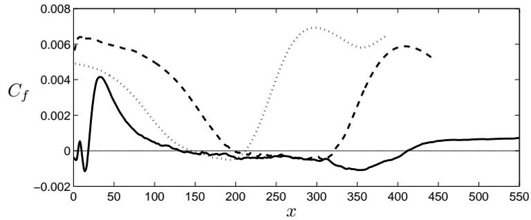
FIGURE 4.3. —  $C_f$  from SEP; --  $C_f$  from Na & Moin (1998);  $\cdots$   $C_f$  from Spalart & Coleman (1997).
