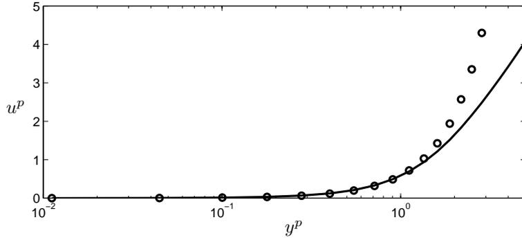
FIGURE 4.12. Velocity profile close to reattachment. — SEP;  $\circ u^p = \frac{1}{2}(y^p)^2$ .
