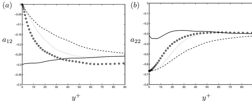
FIGURE 5.2. A3 at  $x = 150$ :  $\circ$  DNS;  $—$  non-damped EARSM; Damped EARSM with the scaled coordinate in  $f_1$  as  $-- y^+$ ;  $\cdots y^*$ . a)  $a_{12}$ . b)  $a_{22}$ .
