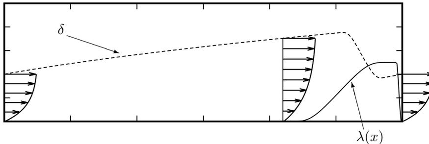
FIGURE 2.1. The boundary layer thickness  $\delta$  (dashed) of a laminar mean flow that grows downstream in the physical domain and is reduced in the fringe region by the forcing. The flow profile is returned to the desired inflow profile in the fringe region, where the fringe function  $\lambda(x)$  is non-zero.
