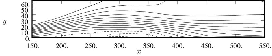
FIGURE 4.11. SEP: contours of mean velocity. Positive values shown as solid lines, negative as dashed.
