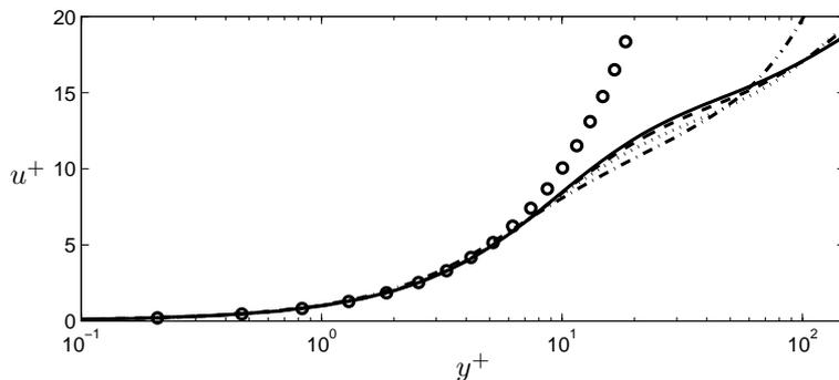
FIGURE 4.8. Velocity profiles at  $x = 300$ . — ZPG; - - A1;  $\dots$  A2; - · - A3;  $\circ$   $u^+ = y^+$ .
